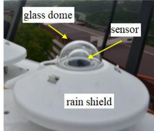
Figure 2: Pyranometer (CMP11) used to measure D_h . A shading ball device is used to block the D_n component, such that only D_h is received by the sensor.
